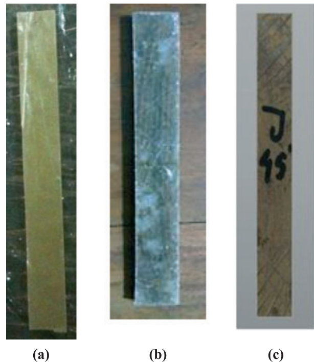
Figure 2. Photographic view of test specimens (a) Glass fiber reinforced composite (b) Glass-jute fiber reinforced composite (c) Jute fiber reinforced composite.
